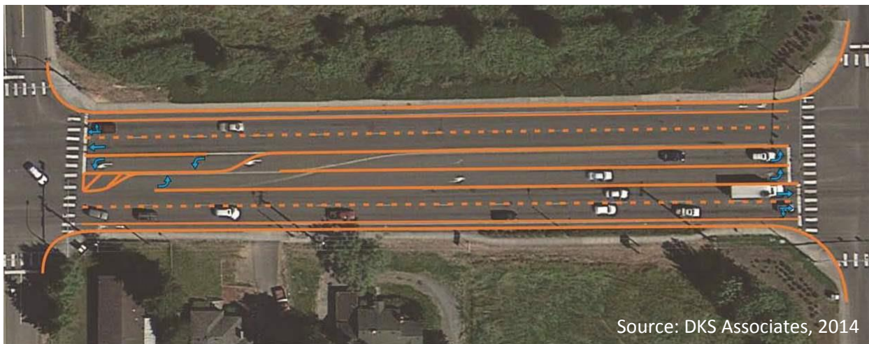
Figure 8. Potential W Main Street Cross-Section West of SR 503 – Option 2 (With Westbound Left Turn Storage Reduction)
