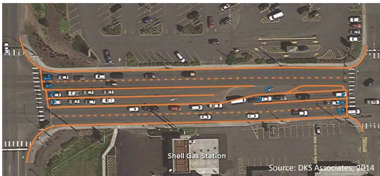
Figure 6. W Main Street Proposed Cross-Section East of SR 503 (With Elimination of Westbound Left Turns into the Shell Station)
