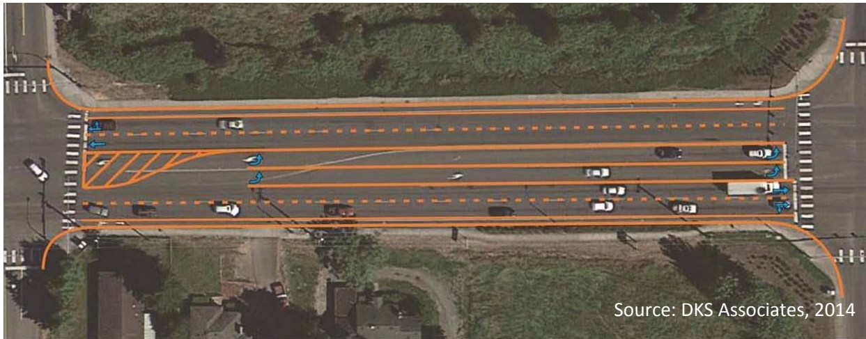
Figure 7. Potential W Main Street Cross-Section West of SR 503 – Option 1 (With Elimination of Westbound Left Turns onto SW 12 th Avenue)
