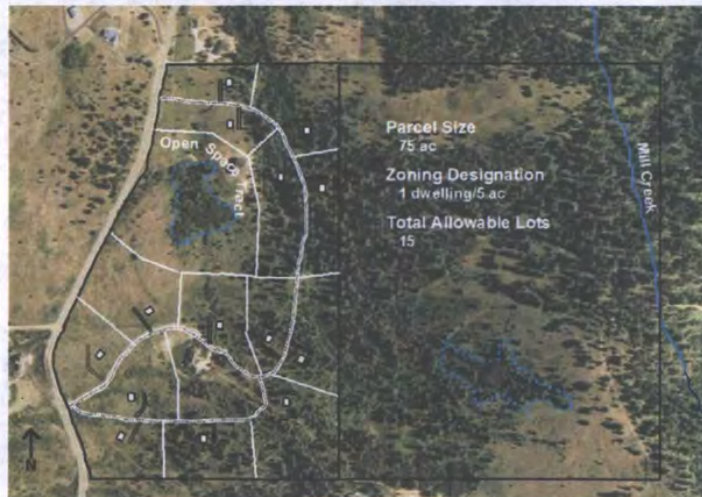
Figure 7.6 Example of a layout that has a slightly lower risk to wildlife (i.e., a limited conservation design) in the western tract. Flexible lot sizes allow for the designation of an open space tract.
