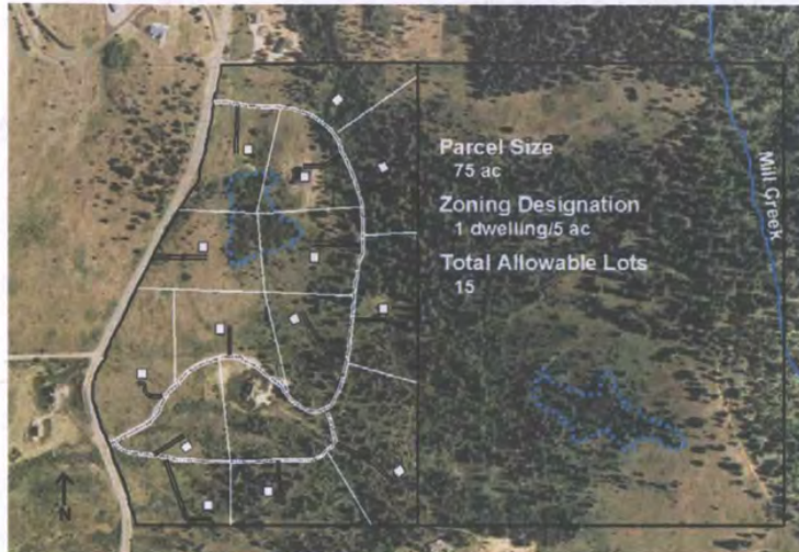
Figure 7.5 An example of a conventional layout for development of the western parcel.
