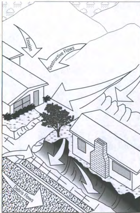
Figure C38. Schematic of an unprotected home , in the path of a debris flow and (or) "mudslide." Suggested methods to reduce the hazards from debris flows are shown in figure C39.
