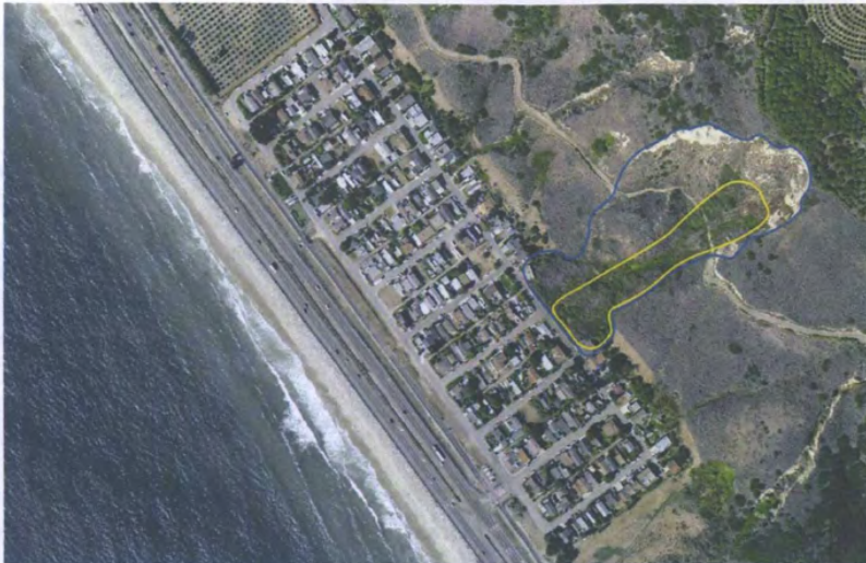
Figure B4. An example of an aerial photograph of the La Conchita landslide in California, USA, taken in 2005. Blue line delineates an older landslide, yellow a more recent landslide. (Photograph courtesy of AirPhoto USA and County of Ventura, California, and Randy Jibson, U.S. Geological Survey.)
